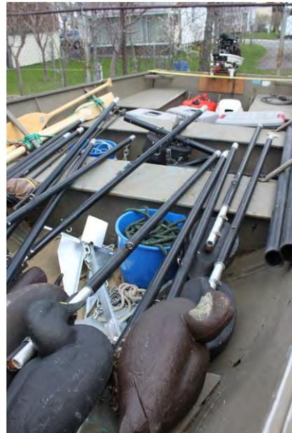
Offshore sets are a bit more difficult to deploy, but it becomes easier with practice. You should first assemble all the hubs and have them on the boat ready to deploy. All lines (anchor lines and tension lines) should be stored so they feed out smoothly; 5-gallon buckets are perfect for storing lines. Essentially, you will start at one end of the assembly (1<sup>st</sup> anchor), and lay out all the other gear in line as the boat backs up slowly.
