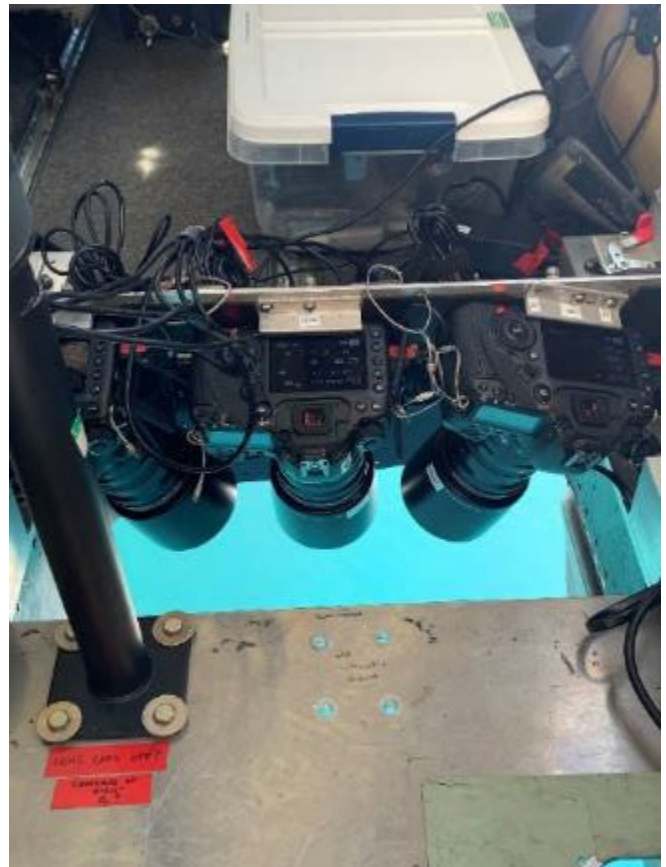
Figure 2. Photo of USGS camera setup in the belly window of a Partenavia.
